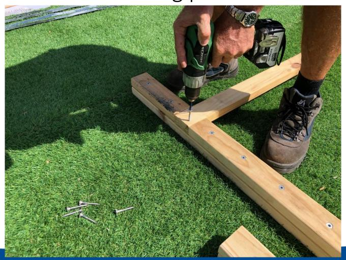
Mark the centre of each leg unit cross member using the short scrap provided in the kit. The distance between the centre support and the side supports is 220mm. Mark each side support as well.
